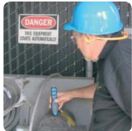
At the same time, the SKF Machine Condition Advisor's non-contact infrared sensor measures the surface temperature of the measurement location and simultaneously displays all three measurement values.
