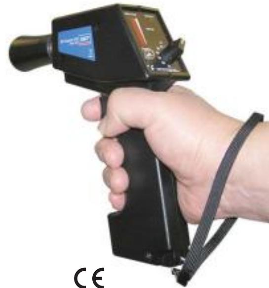
Ultrasonic Probe, a leak can be heard through the headset as a rushing sound or noted on the meter bar graph indicator. The closer the instrument is to the leak, the louder the rushing sound and the higher the meter reading. Should ambient noise be a problem, a rubber focusing probe may be used to narrow the instrument's reception field and to shield it from conflicting ultra sounds.
