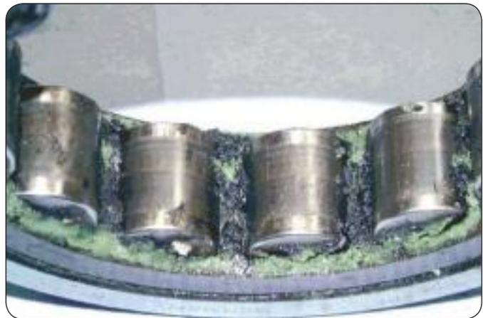
*Lubricant degradation caused by electrical discharge currents.*
